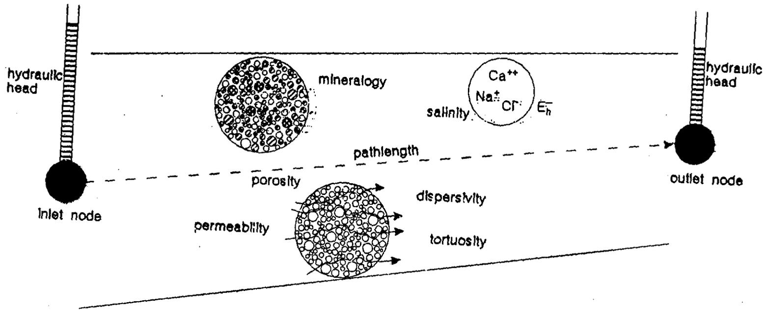
**Illustration of the Principal Properties of a GEONET Transport Segment**
